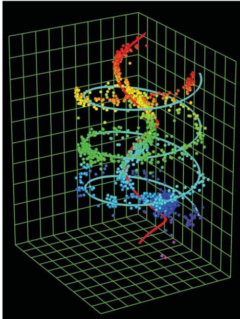
Figure 11: *Two electron tracks from  $^{90}\text{Sr}$  source recorded with the Timepix chip as anode in a 5  $\text{cm}^3$  TPC inside a 0.2T magnetic field.*
