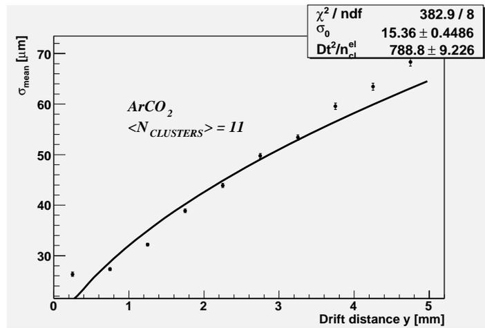
Figure 10: The resolution  $\sigma_{meas}$  as function of the driftdistance in  $\text{ArCO}_2$  for a small pitched GEM
