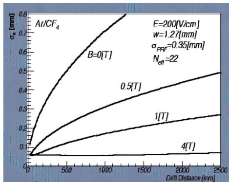
Figure 2: The  $R\phi$  spatial resolution of GEM TPC calculated by the analytic formula for Ar(97%)- $\text{CF}_4$ (3%) gas mixture in the magnetic field up to 4T.
