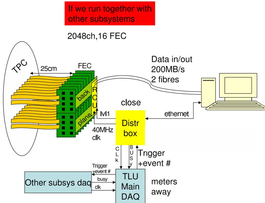
Figure 9: *Layout of the TPC electronics, including hardware and DAQ components.*
