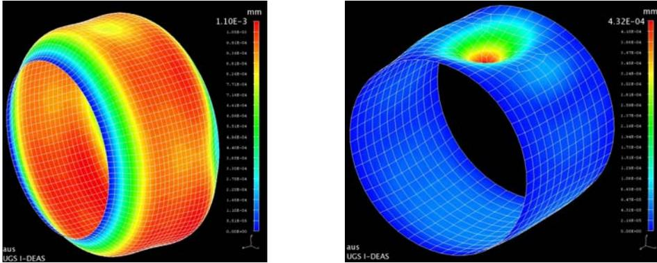
Figure 8: *Left: Result of the simulation of the behaviour of the field cage under an overpressure of 100 mbar. Right: Expected deformation of the field cage under a point-like force of 5 kg at the top.*
