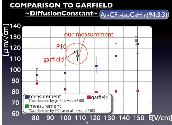
Figure 5: Comparison of  $C_d$  measured by the MP-TPC (blue) in 1T field to the predictions by the Garfield simulation (red) for Ar(94%)-CF<sub>4</sub>(3%)-iC<sub>4</sub>H<sub>10</sub>(3%) with a calibration point for P10 gas (green). The results are still preliminary.
