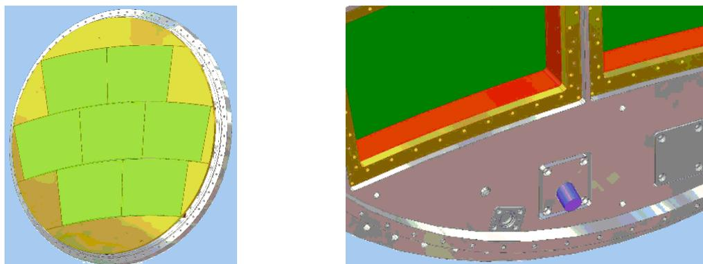
Figure 1: *Left: Design of the large prototype endplate. Right: Detailed view of the endplate with some auxiliary connections and mountings for calibration system.*
