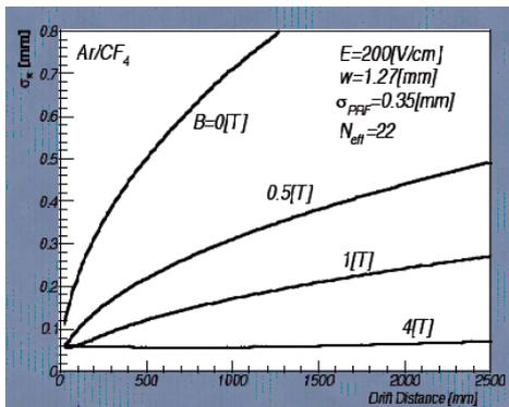
Figure 2: The  $R\phi$  spatial resolution of GEM TPC calculated by the analytic formula for Ar(97%)- $\text{CF}_4$ (3%) gas mixture in the magnetic field up to 4T.
