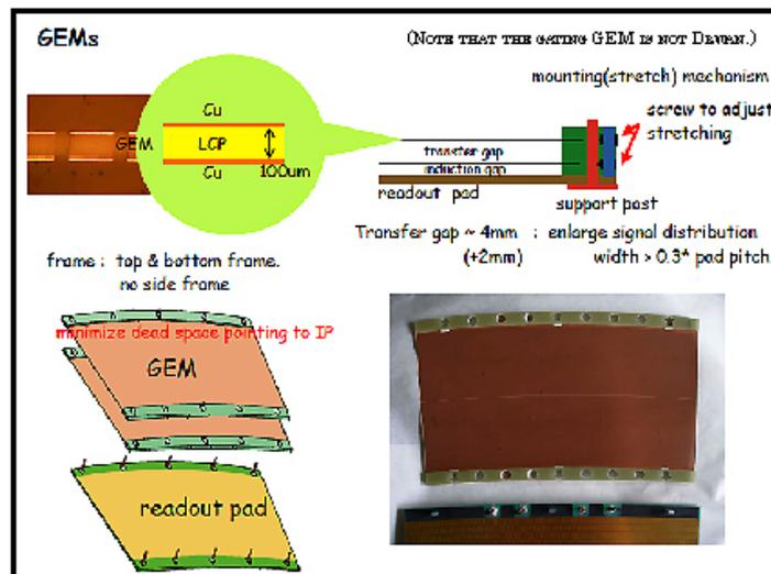
Figure 7: A sketch of the GEM detector module for the TPC Large Prototype test at DESY. The gating GEM on the top of the two 100  $\mu\text{m}$  GEMs for gas amplification is not drawn. The GEMs are supported at the top and bottom frames to minimize the dead area in  $R\phi$ . The GEM voltages are supplied through pins at the frames.
