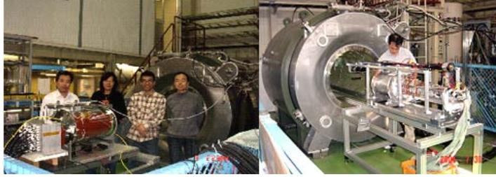
Figure 3: TU-TPC prototype and people from Tsinghua University and KEK in front of the MRI magnet (left), and the same MRI magnet with MP-TPC prototype in the KEK Cryogenic Center.
