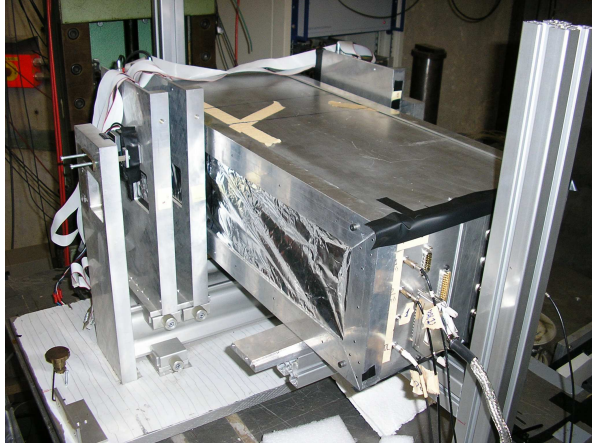
Silicon modules in the Faraday cage inserted in between the beam telescope at DESY
