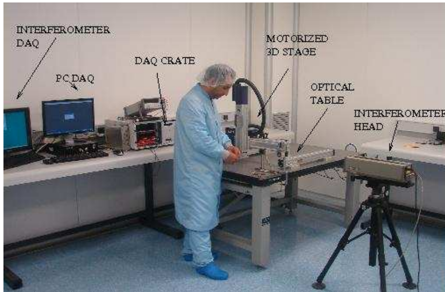
Components used for optical characterization and scanning of transparent Si microstrip- detectors
