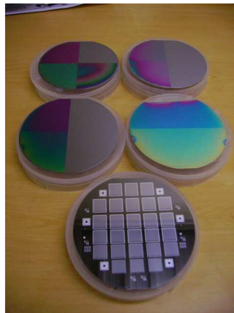
Top left: Undoped Si with SiO 2 and Si 3 N 4 . Left to right, top to bottom: same as before but with increased doping level. Bottommost sample contains small samples of microstrip detectors
