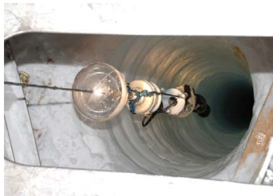
Fig. 4.3 Pinger moving down a hole
