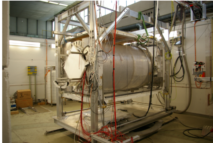
FIGURE 2.7. Movable stage in test beam area.
